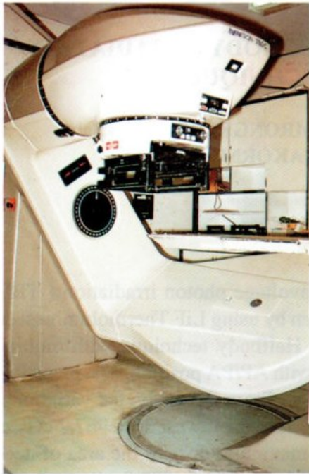
Fig.1 Treatment geometry of Cobalt-60 unit in small therapy room (170 cmSSD)
